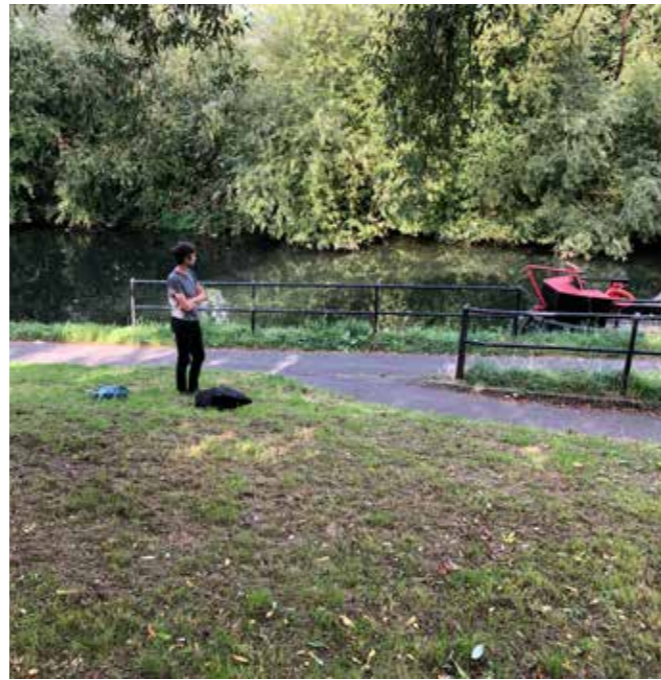
Reducing the length of the handrail will allow for the landing of the ramp to be widened, providing better access to the towpath.
